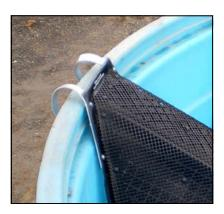
Try not to make the bend directly on the bolt hole. Use Vice Grips to help position the bend. Tip: If straps are very cold, heating the bending zone can make it easier to bend.
