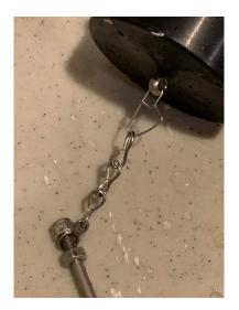
The float assembly has been pre-adjusted for an average water level. If you want to adjust the water level, it's easiest and more accurate to do so by changing the clip up or down on the chain.
